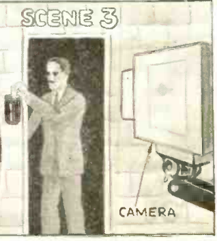
Camera No. 1 shifts to actor in full-size door, and takes up action when door image in Scene 2 has been "panned up" to full size.
